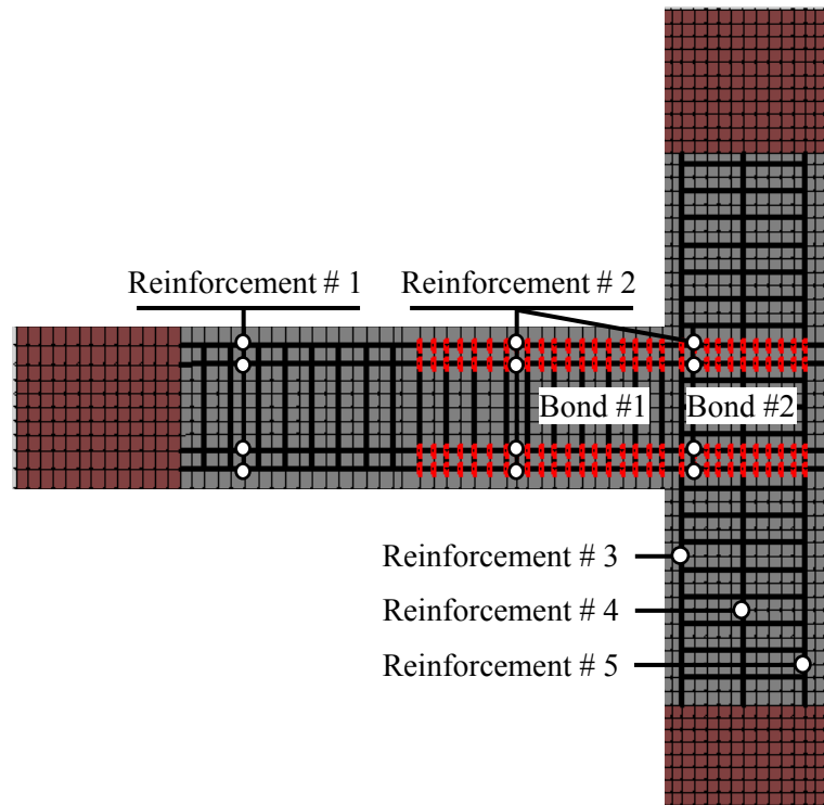
Fig. 3.13 Reinforcement and Bond Regions for Specimen ED2
