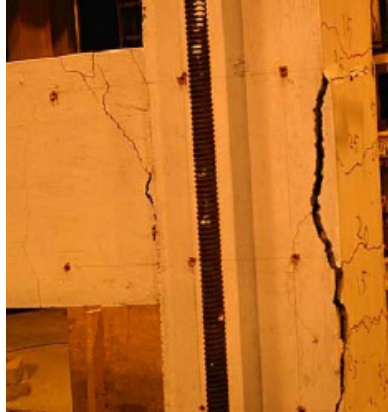
Fig. 3.30 Final Failure at the back side of Specimen TDD1 (from Chen, 2006)
