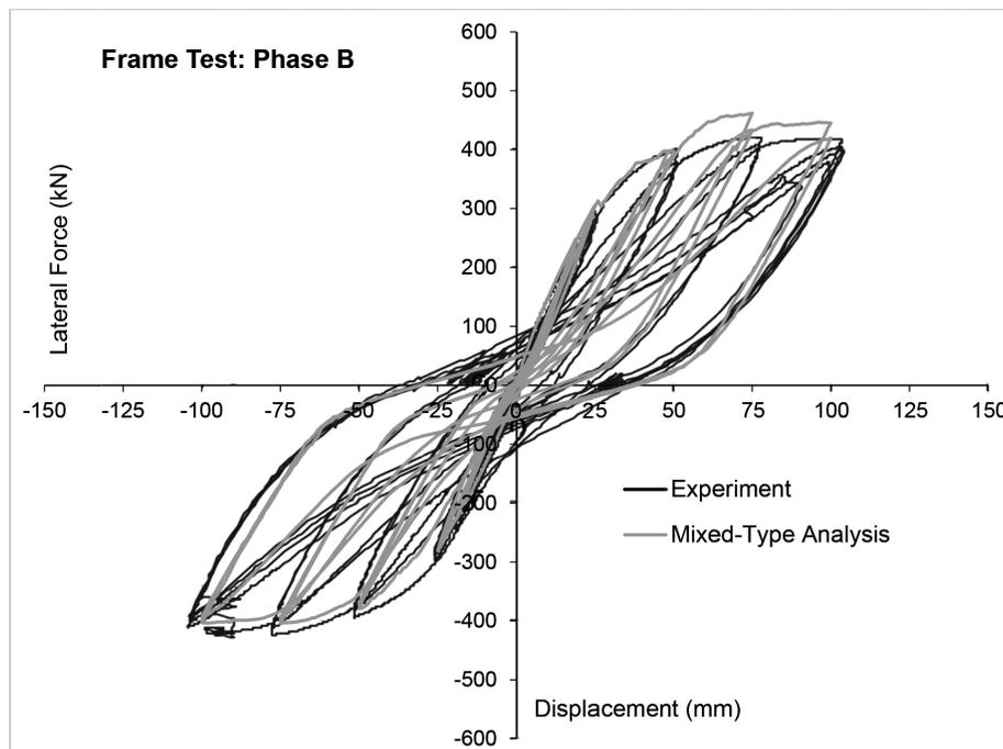
**Fig. (7).** Load-deflection response of experiment and mixed-type analysis for Phase B.
