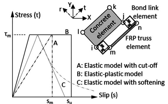
Fig. (2). FRP link element and different types of stress-strain relationship for bond.
