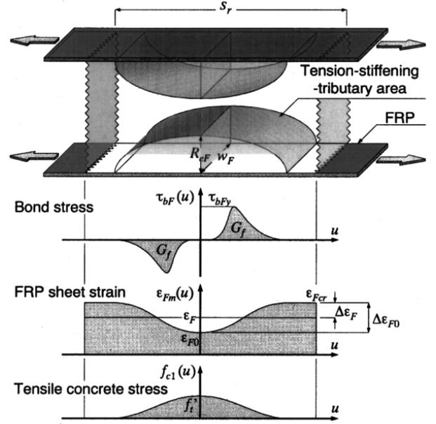
Fig. (3). Tension stiffening effects of FRP sheets [33].
