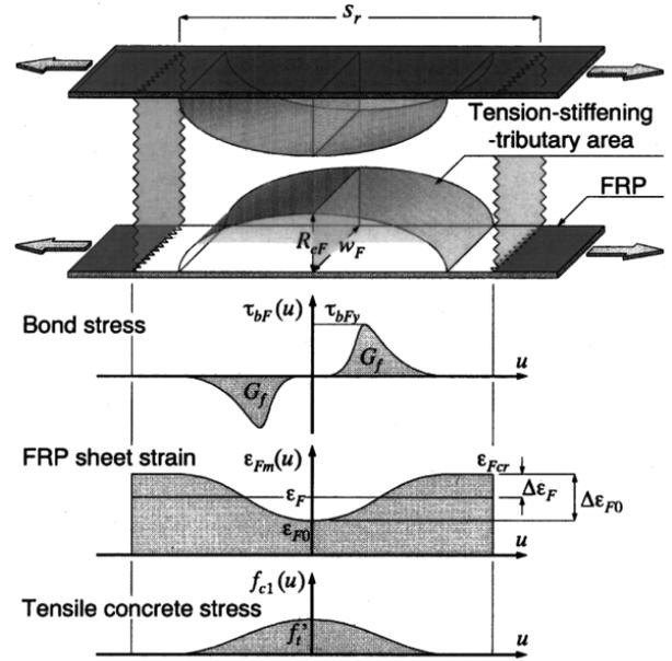
Fig. (3). Tension stiffening effects of FRP sheets [33].
