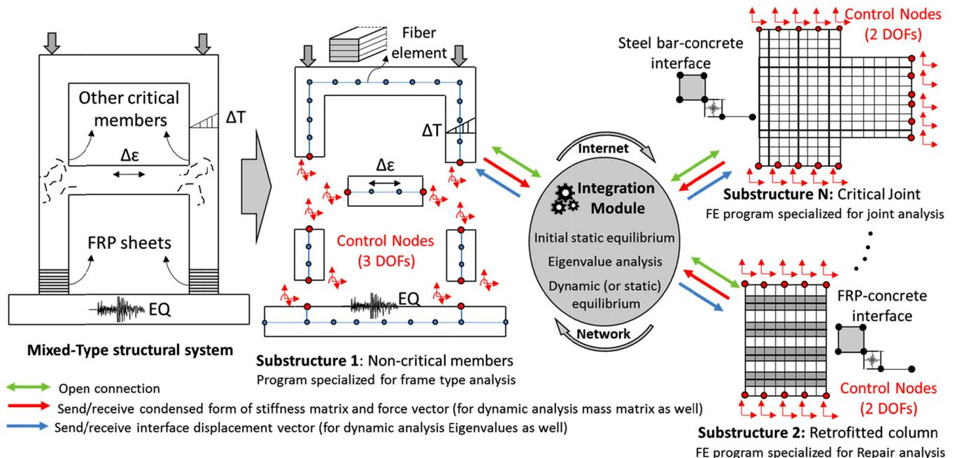
Fig. (1). Overview of the proposed multi-scale analysis approach.
