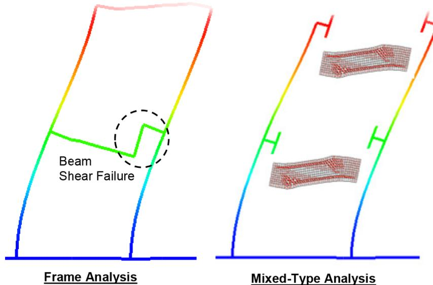
Fig. (6). Crack pattern and deflected shape of the frame.
