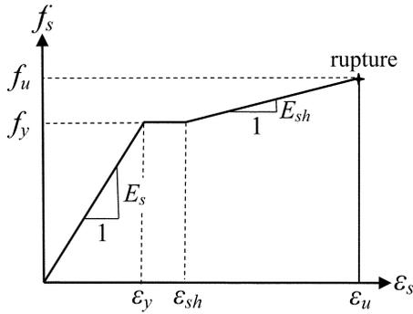
Fig. 10—Trilinear stress-strain relationship for reinforcement.
