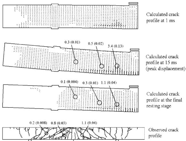
Fig. 9—Observed and calculated crack profiles, SS3a-2. (Note: Crack widths in mm [in.] )
