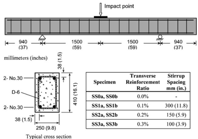
Fig. 2—Specimen properties.
