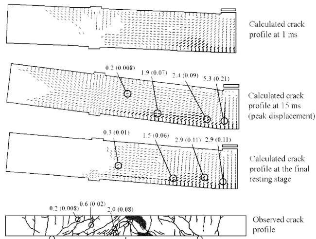
Fig. 10—Observed and calculated crack profiles, SS2b-2. (Note: Crack widths in mm [in.] )
