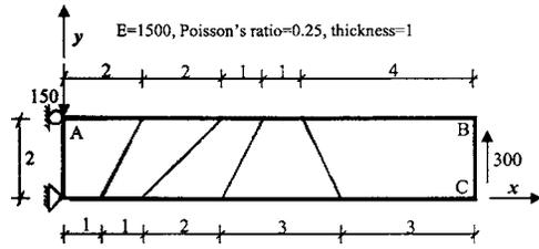
Fig. 2. Problem 1: cantilever beam under end shear
