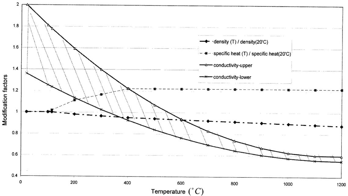
Fig. 1 Modification factors: thermal-analysis-related properties
