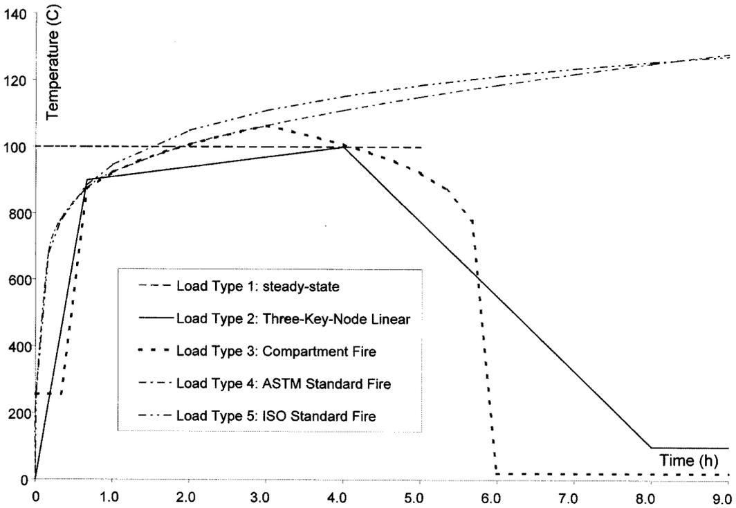
Fig. 12 Various thermal loads tested in Problem 3
