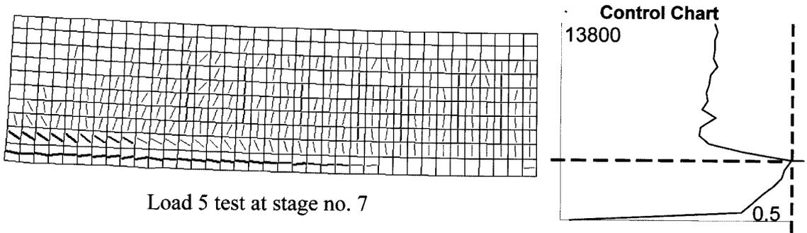
Fig. 14 Crack pattern in load 5 test in Problem 3
