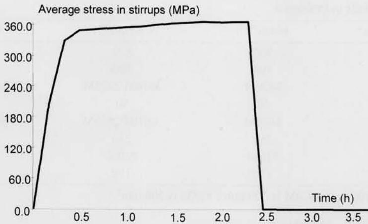
Fig. 15 Average stress in stirrups in load 4 test in Problem 3
