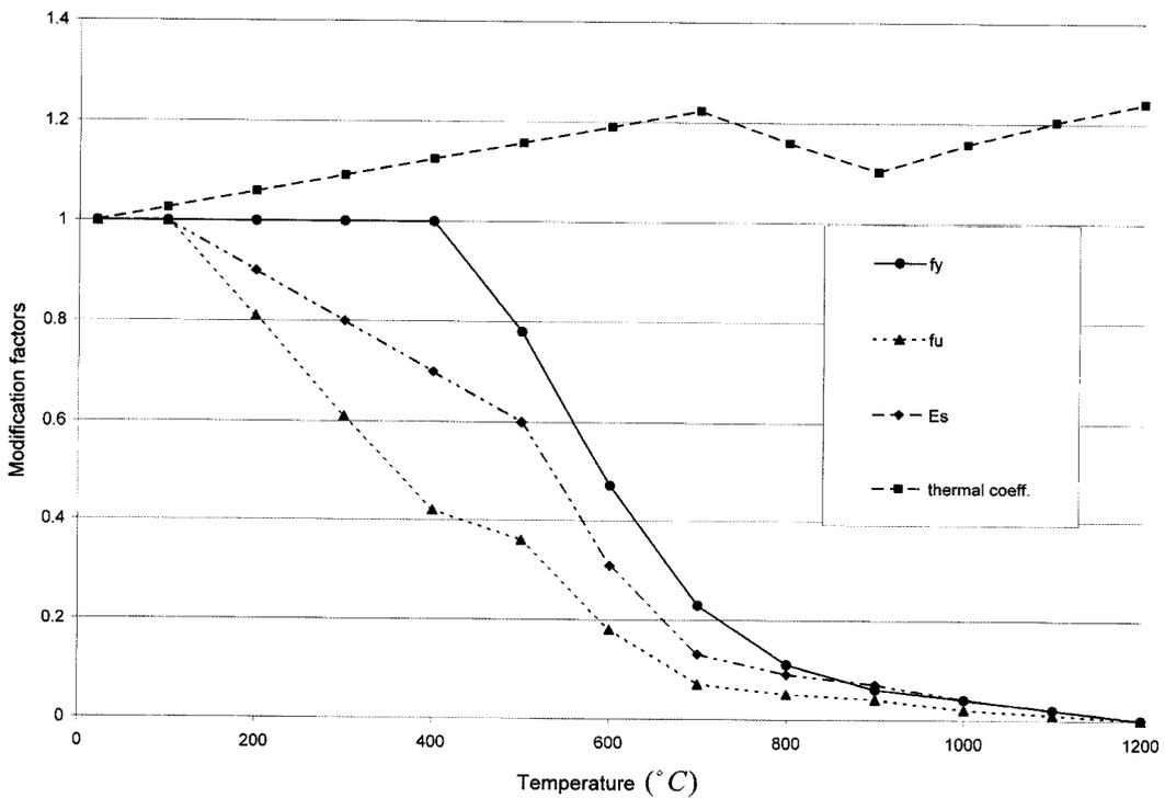
Fig. 3 Modification factors: steel's structural-analysis-related properties
