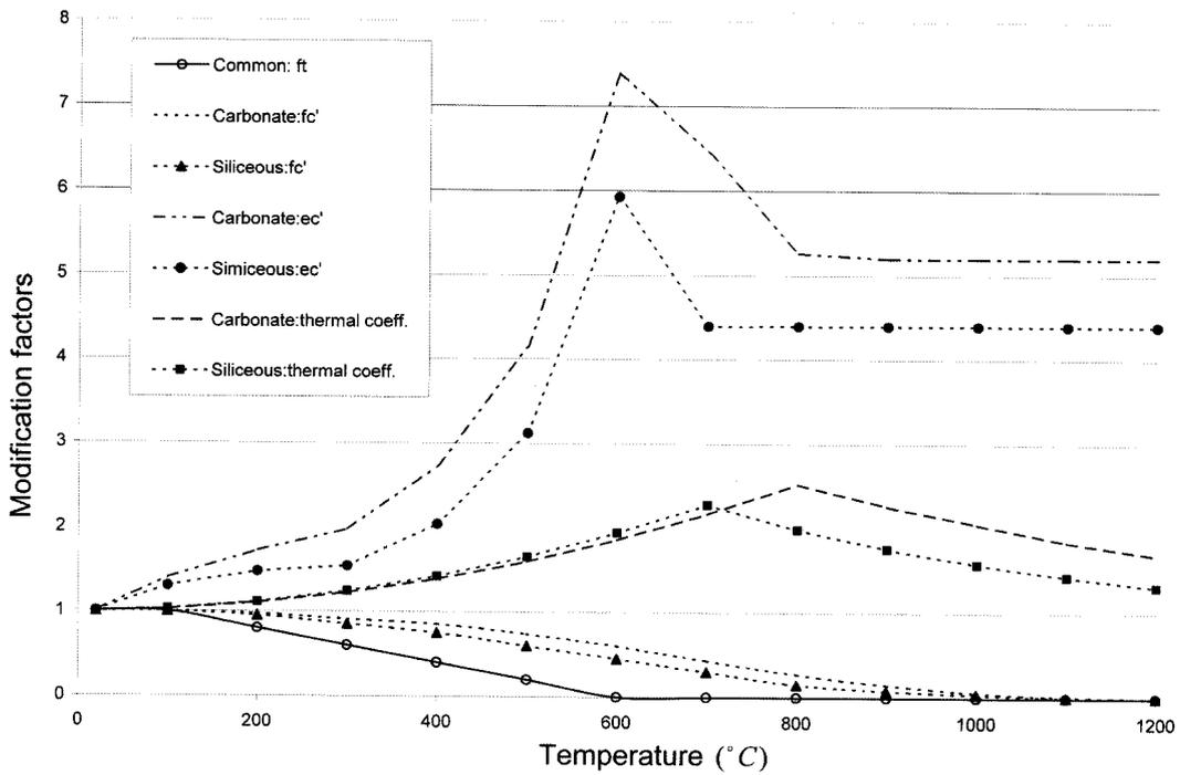
Fig. 2 Modification factors: concrete's structural-analysis-related properties
