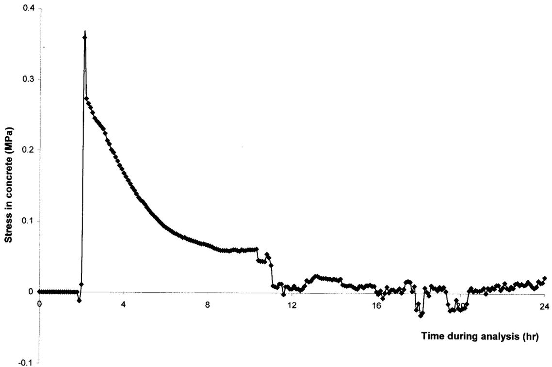
Fig. 19 Typical primary concrete stress in Type I test in Problem 4
