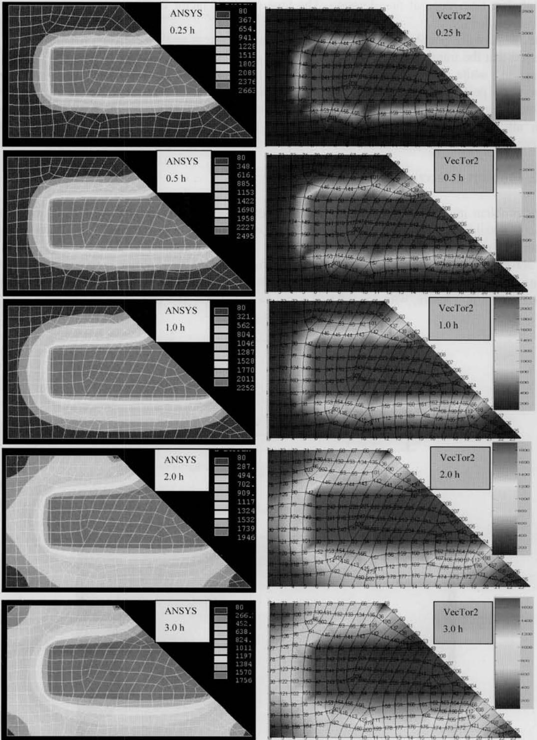
Fig. 9 Temperature contour plots in Problem 2
