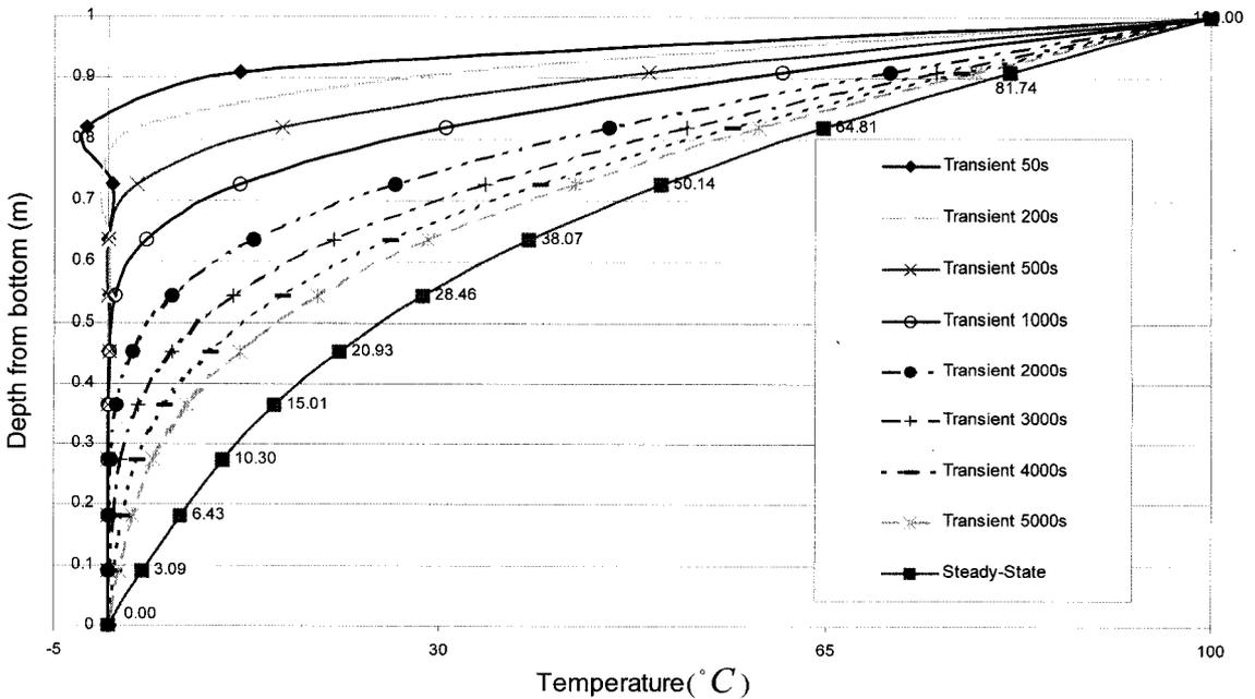
Fig. 6 Temperature profile through the depth of the cross section in Problem 1
