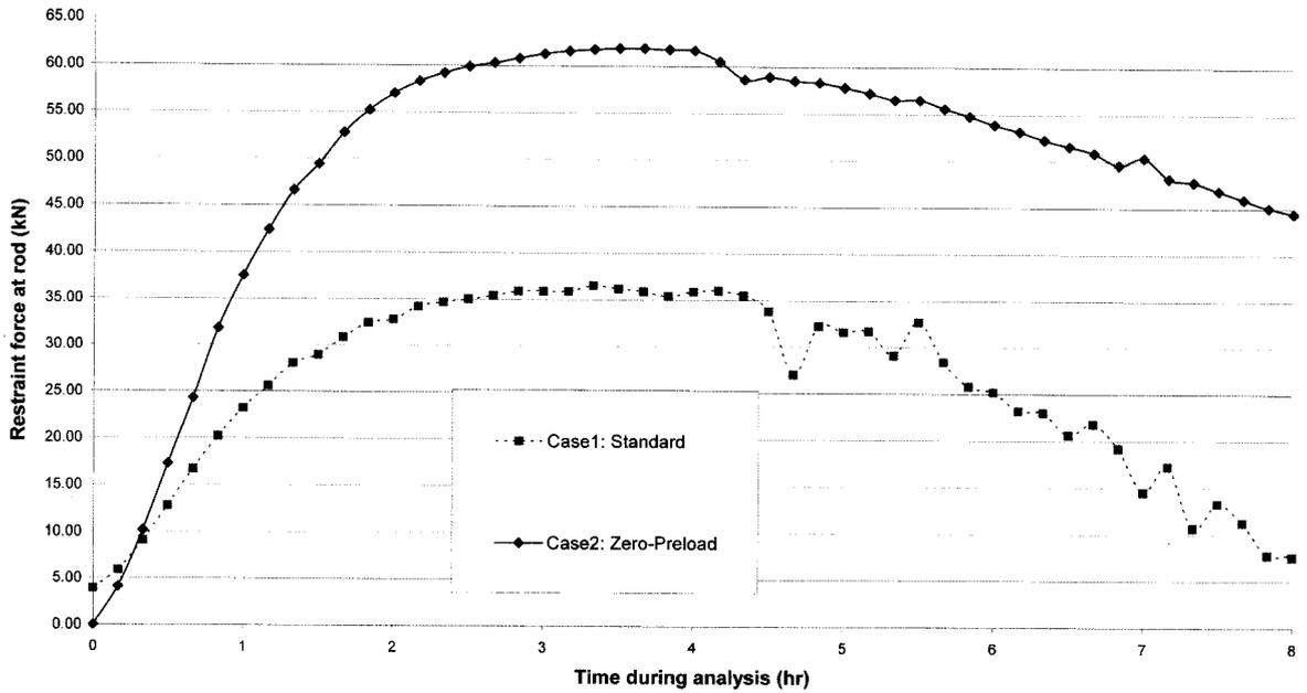
Fig. 20 Restraint force induced at engaged tie-rods in Type II test in Problem 4
