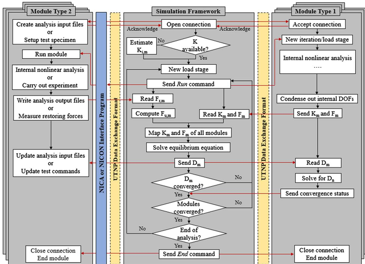
Fig. 2. Algorithm of the proposed multi-platform framework.
