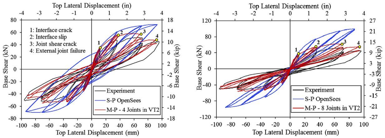
Fig. 8. Load-deflection responses of frame for reversed cyclic analyses of Type A models (left) and Type B models (right).
